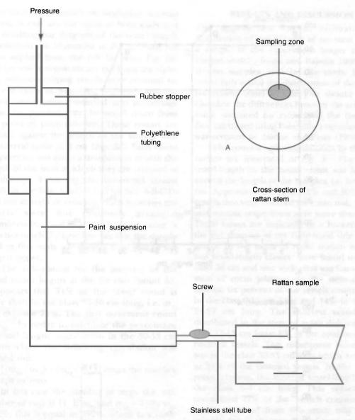
Fig 1. Schematic diagram of the apparatus used to infuse alkyd-paint into a rattan sample. A: The paint applicator is tapped into the shaved end near the periphery of the rattan stem for random sampling
